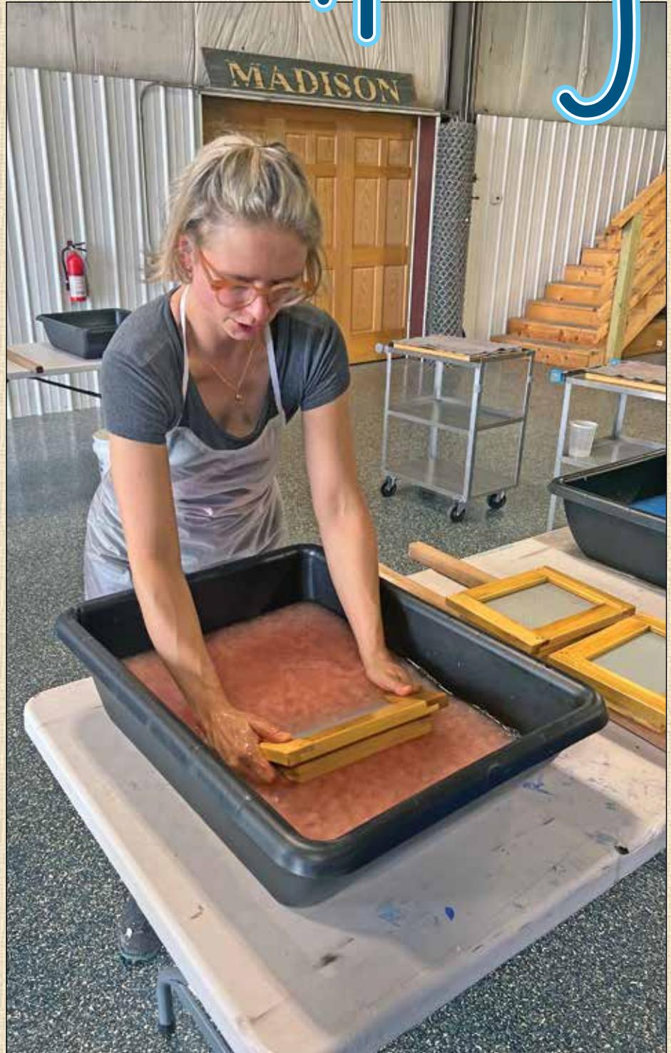
The screen is dipped in the softened fiber to create a sheet of paper.
