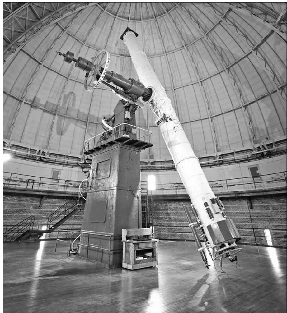
above: The telescope that makes its home in the observatory was the largest operating telescope in the world from 1897 to 1908. The dome where it resides is 112 feet high and 90 feet in diameter. The telescope itself is 64 feet long. top: Yerkes Observatory has experienced a series of upgrades, including the installation of solar panels, at its Williams Bay complex, the expansive footprint of which can be seen via this photograph from above.
